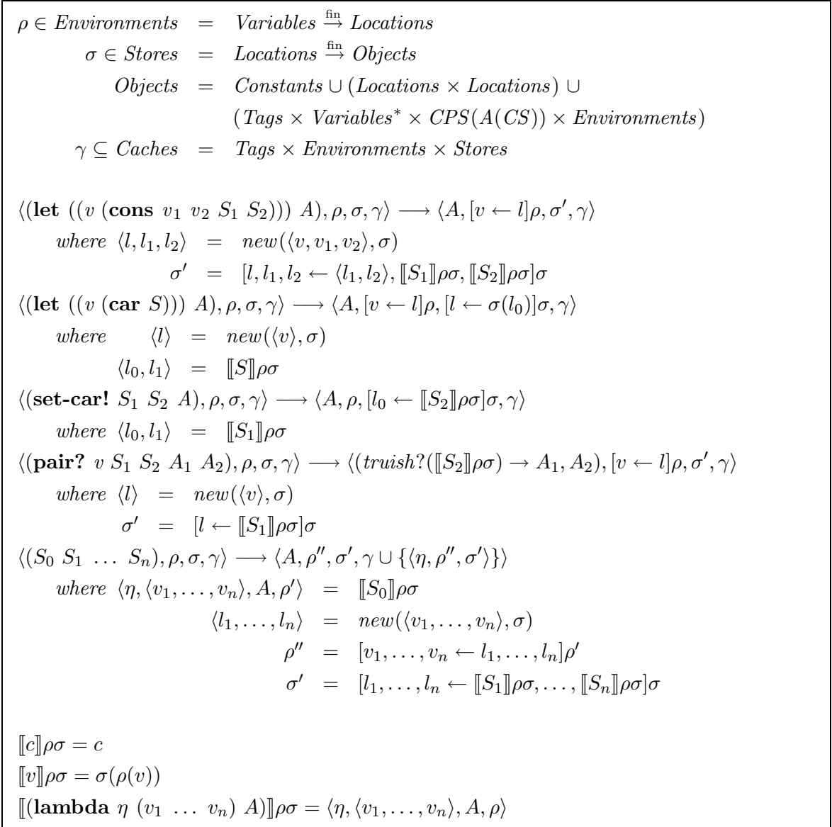
Figure 4.1: Domains and transition relation for the collecting machine.
